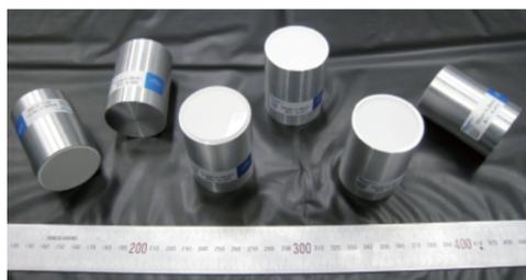
LaBr<sub>3</sub> crystals (2.0 inches long, 1.5 inches in diameter)
