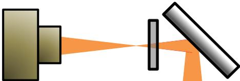
A schematic diagram showing a CCD camera 1 with a microscope objective lens. An orange beam of light is focused through the objective lens onto a small rectangular component, likely a sample or detector.
