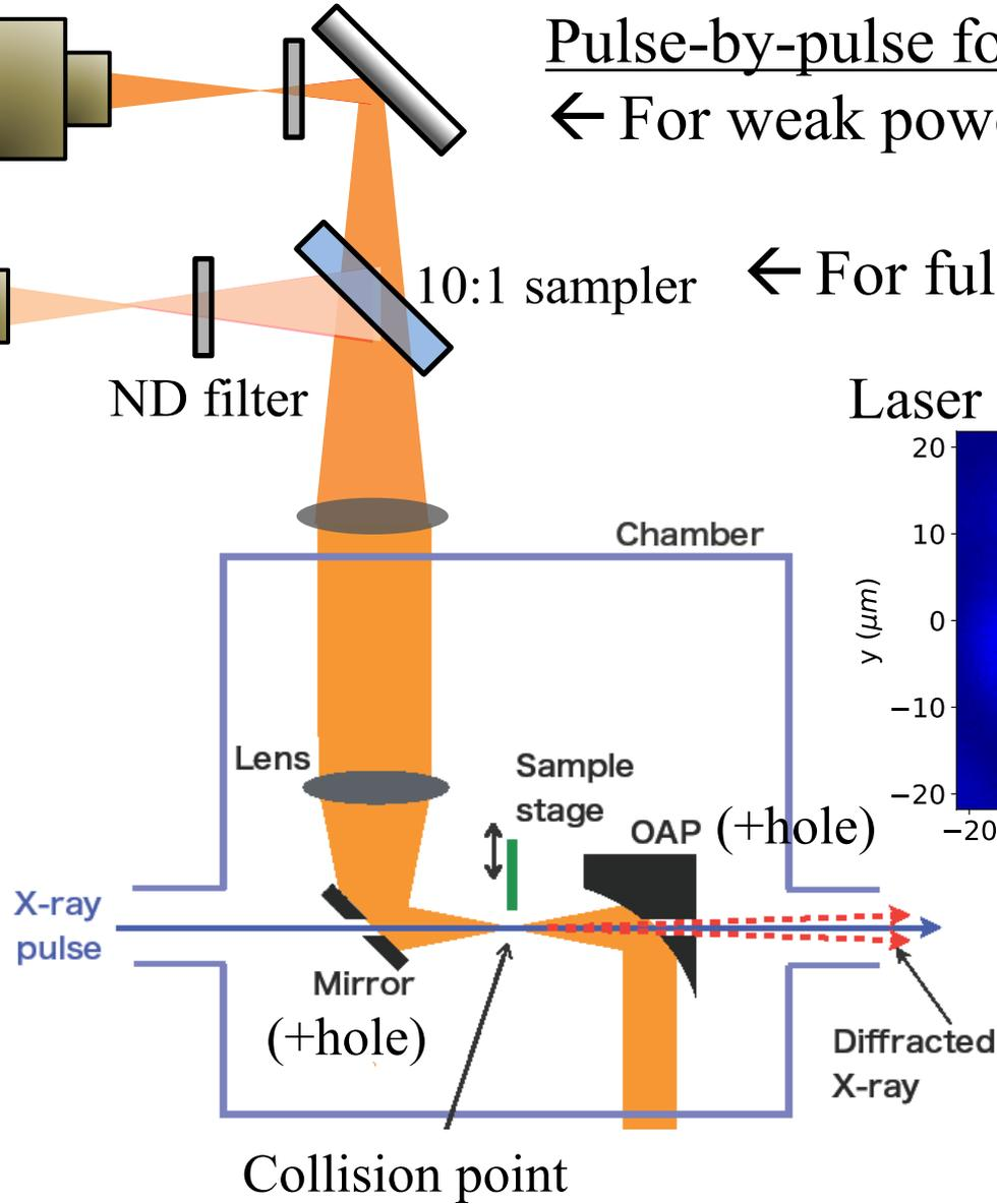
Laser focal size  $\sim 10 \mu\text{m}$
