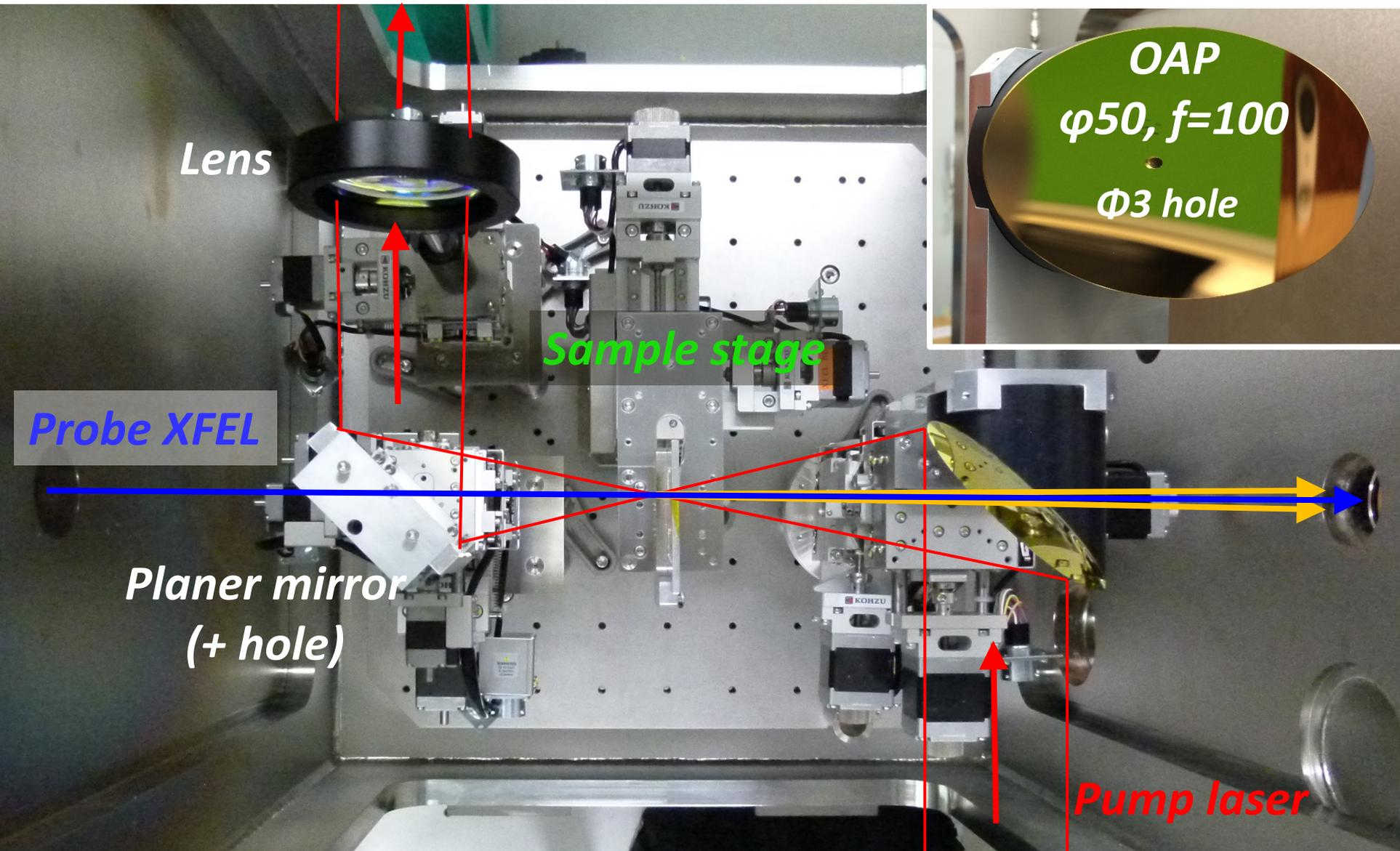
Many stages with motors to adjust the focal position and its size
