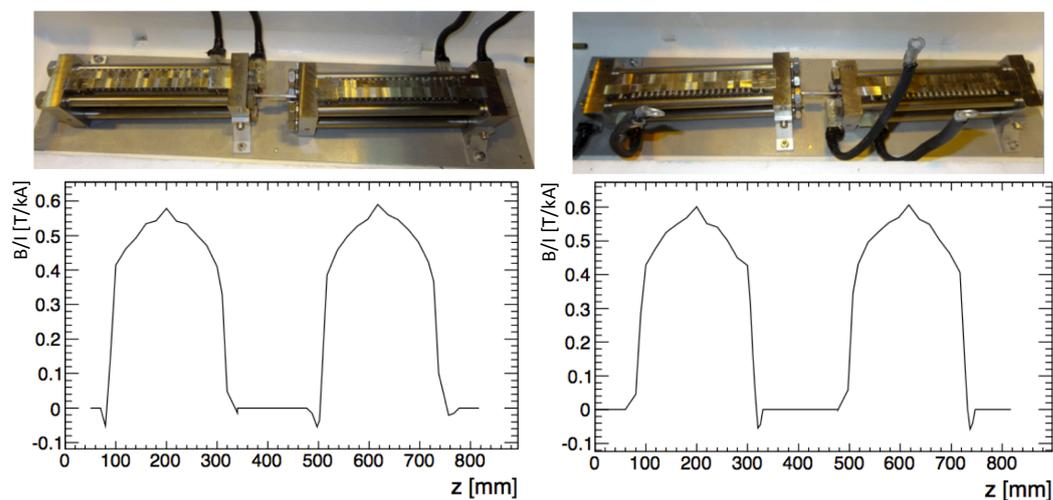
Figure 4.6: Field maps of the upstream ( $I_u$ , left) and the downstream ( $I_d$ , right) regions. The spacing between the two magnets is  $417 \pm 1$  mm. The maps are scaled from Fig. 2.11 using field-current ratio at high voltages shown in Fig. 2.7.
