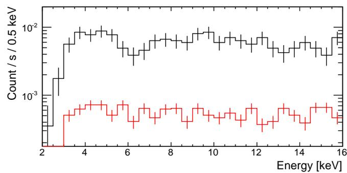
Figure 3.17: Measured background energy spectra. The energy threshold is set around 3 keV. The black/red spectrum is obtained without/with the outer shield, respectively. The shield reduces the background rate by a factor of more than  $10^{-1}$ .
