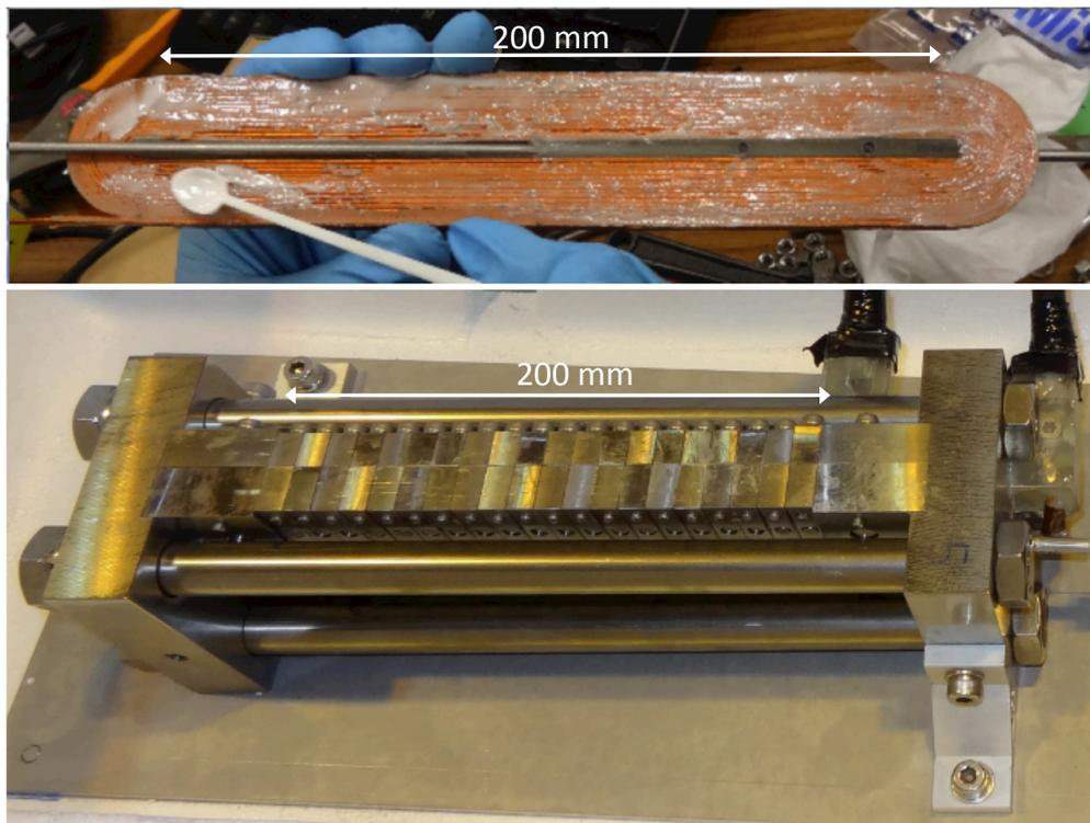
Figure 2.2: Pictures of the magnet. Top: a bare coil of Cu wire wound around a GFRP bobbin. Its straight section has a length of 200 mm. The beam pipe diagonally passes through the center of the coil. Bottom: the fully backed-up magnet. The bare coil is backed up with 20 divisions of stainless-steel metal and is compressed in the longitudinal direction by two thick plates with M20 bolts and nuts.
