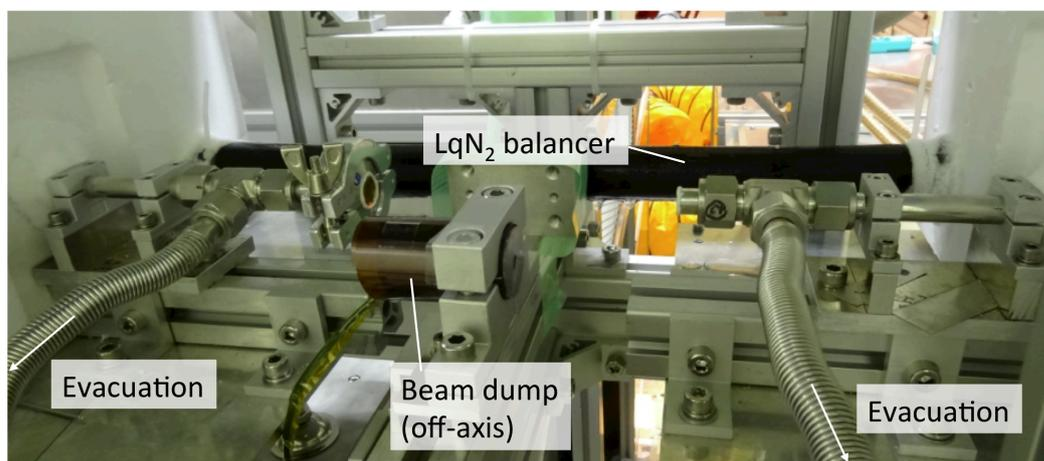
Figure 3.12: Central space below the CT. The beam dump is placed at the center. There are X-ray windows of polyimide with a thickness of  $12.5 \mu\text{m}$ . The air of conversion regions is evacuated near these windows with a scroll pump. Behind these components, a surface level balancer for liquid nitrogen is placed.
