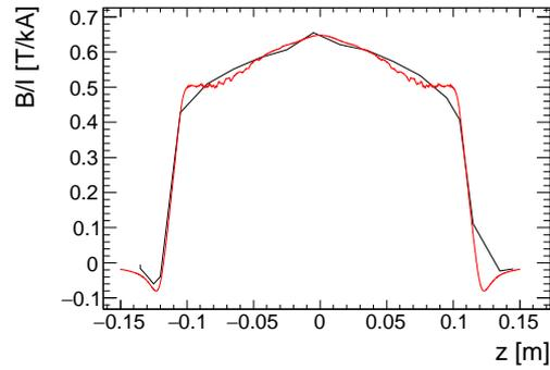
Figure 2.10: Comparison of the measured map (the black line in the right of Fig.2.9) and the calculation of finite element simulation (ANSYS). The simulation includes all the 3D geometrical information. Unsmooth structure at the edges of the simulation reflects the finite size of the mesh. Inhomogeneous distribution of permeability in the backup metal is considered to cause the difference from the measurement. The difference of the area between the two maps is 0.2%.
