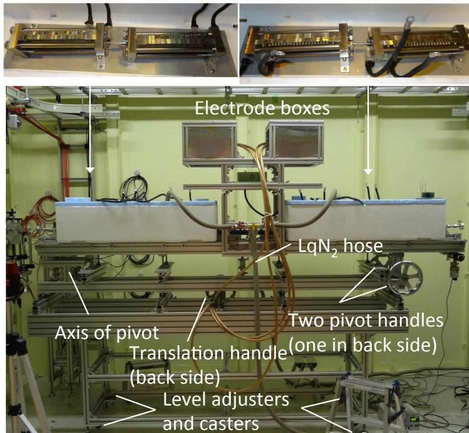
Figure 3.10: Base table of the magnets. It has five-axis alignment mechanism other than the translation along the beam direction. Three of them including the height is realized using level adjusters on its foot. Linear guide rails are used for another translation, which transversely crosses the beam axis. Swing of the base axis applies pivot mechanism.
