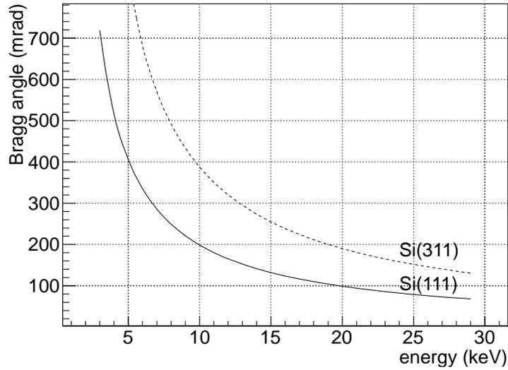
Figure 3.4: Bragg angle as a function of the X-ray energy, calculated with the Bragg condition of  $2d \sin \theta_B = \lambda$ , where  $d$  the lattice spacing of silicon ( $d_{111} = 3.14 \text{ \AA}$  and  $d_{311} = 1.64 \text{ \AA}$ ).
