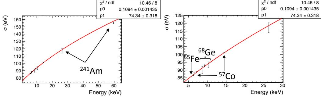
Figure 3.18: Measured resolution as a function of the energy. The data points are fitted with a function of  $\sigma = \sqrt{F W E + \sigma_0^2}$  (see the text). The energy resolution at 9.5 keV is obtained as 93 eV.
