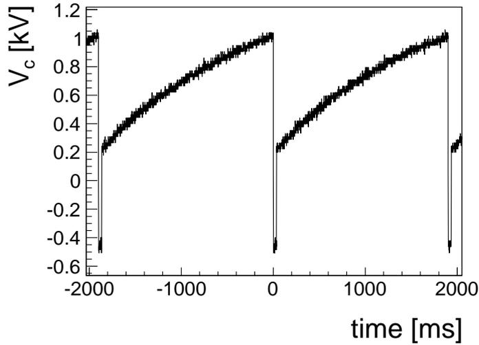
Figure 2.19: Measured time variation of the capacitor voltage with a shot repetition of 0.5 Hz at 1 kV. The voltage is reversed after the first pulse, and then reversed again after the succeeding second pulse. Right after that, an additional charging starts until the voltage returns to its original value.
