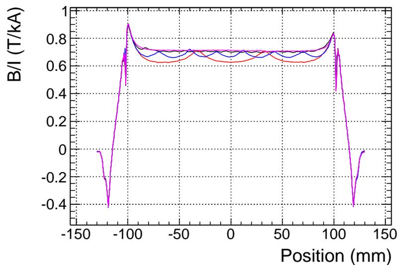
Figure 2.3: Field efficiency with divided backup along with the beam path calculated with 3D finite element simulation. The colored lines show the number of divisions: three (red), seven (blue), 19 (black) and 41 (magenta). The increase of the divisions clearly contributes to the decrease of the field cancellation from eddy current.
