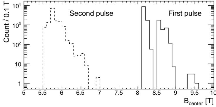
Figure 4.1: Field distribution of the most downstream magnet for the total 13,838 shots. The field is represented by a value at the center of the magnet. The first pulse is ranging from 8.1 T to 9.6 T, and the second pulse is from 5.5 T to 6.9 T. Due to heat loss of the first pulse, the second pulse is generated with a relatively smaller energy. This results in a decrease of the peak field of the second pulse.
