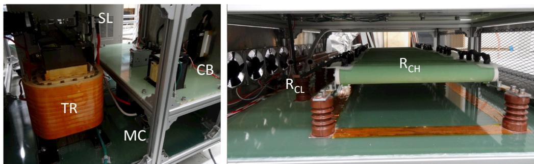
Figure 2.21: Lower floors. Left: the first floor. The transformer (6 kV, 20 kVA) is seen in front of the left picture. Behind it is the slidac with 20 kVA. Right: the second floor.  $R_{CL}$  is composed of 6 k $\Omega$  resistors connected with 2p2s.  $R_{CH}$  is, on the other hand, composed of 16 resistors of 900  $\Omega$  and 700 W each, connected with 4p4s.
