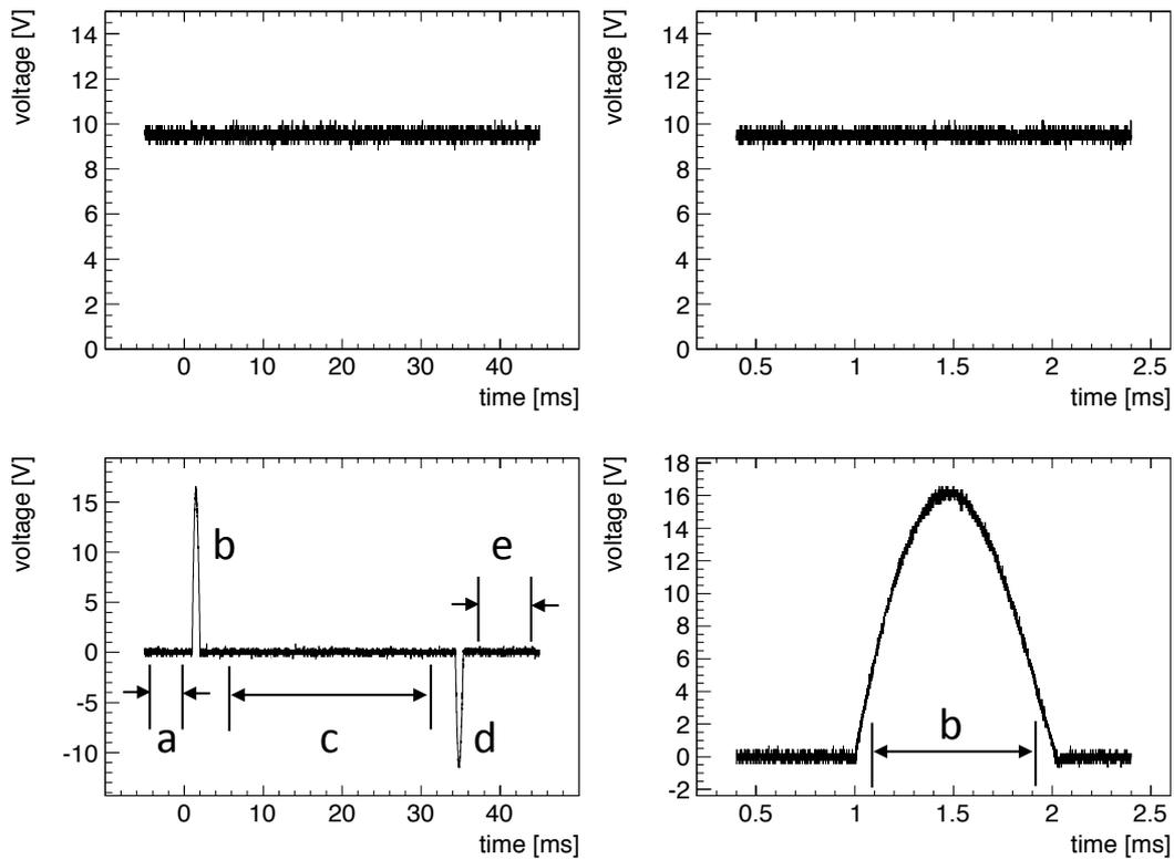
Figure 2.16: Output of the laser power meter during the oscillation test. The gain of its amplifier is adjusted to output 10 V for an input laser power of about 1 mW. The top left figure is its output, and the bottom left figure shows the corresponding current. The pulse interval is set to 33 ms. The top right figure is the magnified view around the first pulse, and the bottom-right figure shows the corresponding current. Significant change is not measured.
