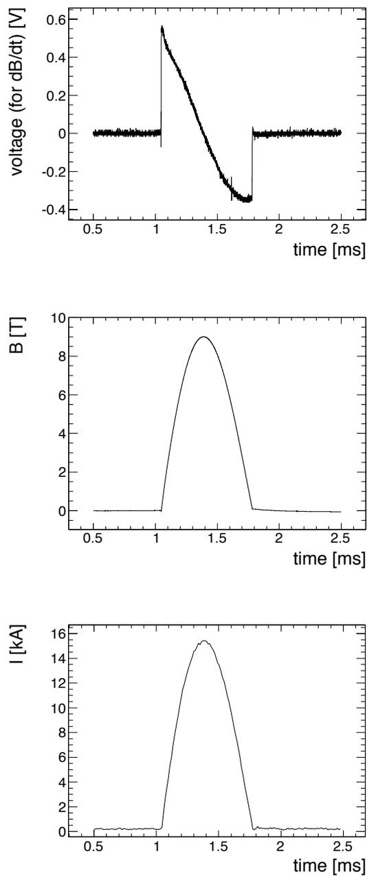
Figure 2.6: Typical shapes of the measured field and current with 2.75 kV. Top: a raw signal of the pickup coil, which is an induced voltage of  $d\Phi/dt$ . Middle: the field shape obtained by an integral of the raw signal. Bottom: the current shape measured with the CT.
