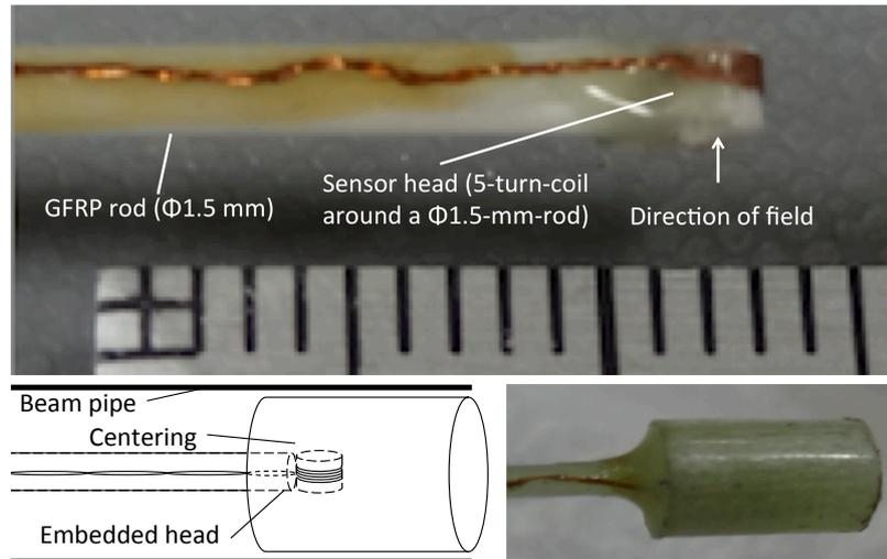
Figure 2.4: Pickup coil. Top: Cu wire ( $\phi 0.1$  mm) coated with enamel ( $t 150 \mu\text{m}$ ) is wound around a GFRP rod ( $\phi 1.5$  mm) with five turns. Bottom: a centering used to measure the field at the center of the pipe. The head of the pickup coil is embedded into the GFRP centering.
