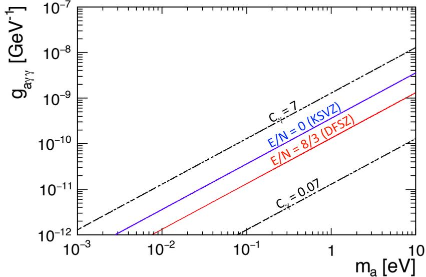
Figure 1.1: Bounds of invisible axion models between the axion-two-photon coupling constant and the axion mass. The blue line is standard KSVZ model ( $E/N = 0$ ), and the red line is DFSZ model ( $E/N = 8/3$ ). The broken lines show the region of typical invisible models with  $C_\gamma$  of 0.07–7, which is referred to as the “invisible band”.
