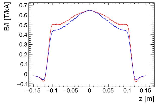
Figure 4.9: Uncertainty from the deviation of the beam path. Maps of the path through the pipe center (red) and the worst path (blue), which deviates from the path through the pipe center by 2.0 mm. These two integrals give their difference of 6.4%.
