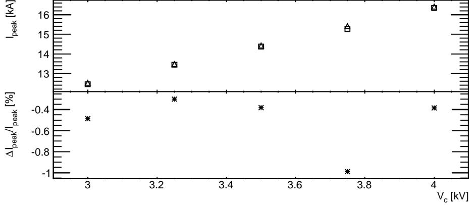
Figure 4.7: Ratio of the two currents ( $I_u/I_d$ ) as a function of charged voltage. Top: the measured currents of the upstream (triangle) and the downstream (box) magnets. Bottom: the difference of the two currents. Their difference is less than 1%.
