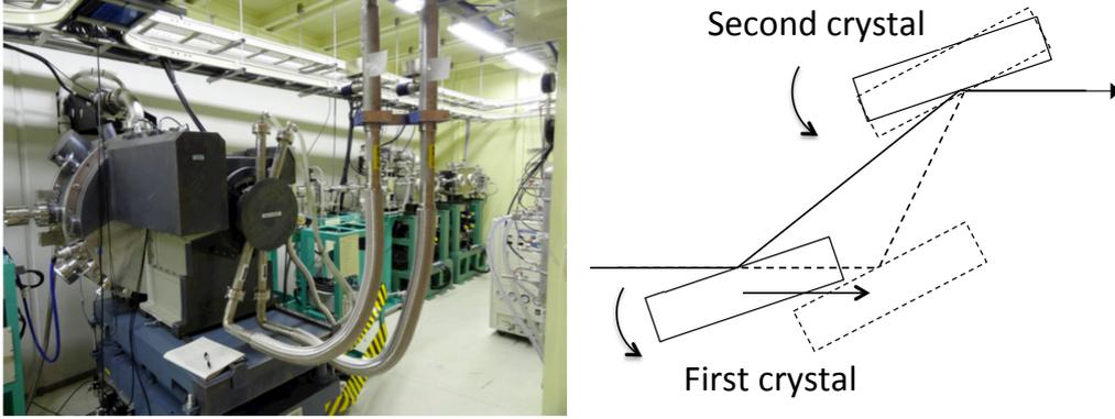
Figure 3.3: Double crystal monochromator (DCM). Left: inside of the DCM is evacuated, and the crystals are cooled with liquid nitrogen due to heat load of the beam. The two metal hoses, in which the liquid nitrogen flows, are shown in front of the left figure. Right: translation movement of the first crystal as well as rotations of the both. In this way, height of the outgoing beam does not change with the energy.
