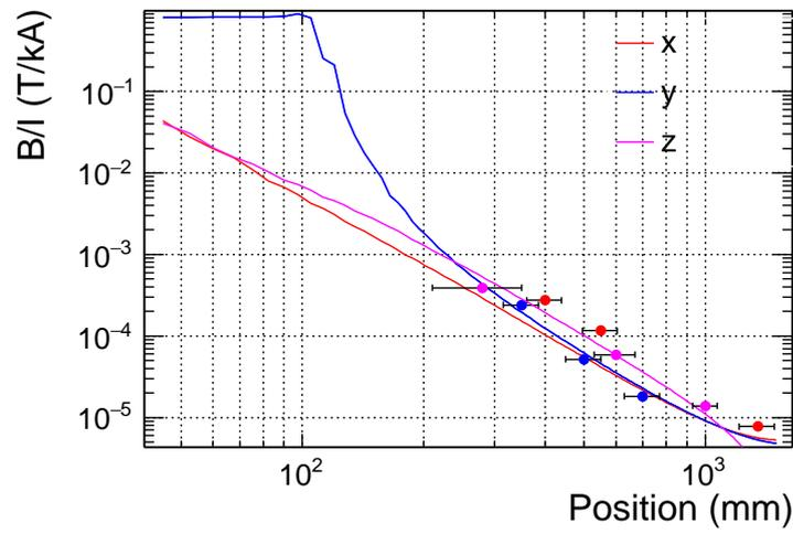
Figure 2.15: Measured magnitude of leakage field in three directions from the center of the prototype magnet. The measurement is carried out with a charged voltage of 1.0 kV and capacitance of 1.6 mF. Results of 3D finite element simulation is also shown with the corresponding line color.
