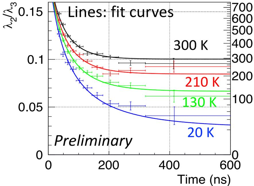
Thermalization curves of Ps in various silica temperature
