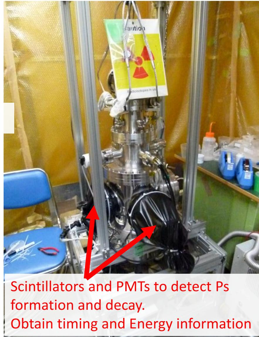
Scintillators and PMTs to detect Ps formation and decay.
