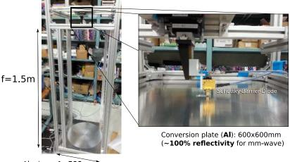
Al mirror  $\Phi = 500$ mm, surface accuracy << 1mm
