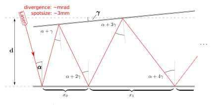
$$\gamma = \frac{\Delta x}{4d\cos\alpha} \lesssim \frac{1\text{mm}}{4 \cdot 1480\text{mm} \cos(10^\circ)} \sim 2 \times 10^{-4}$$
