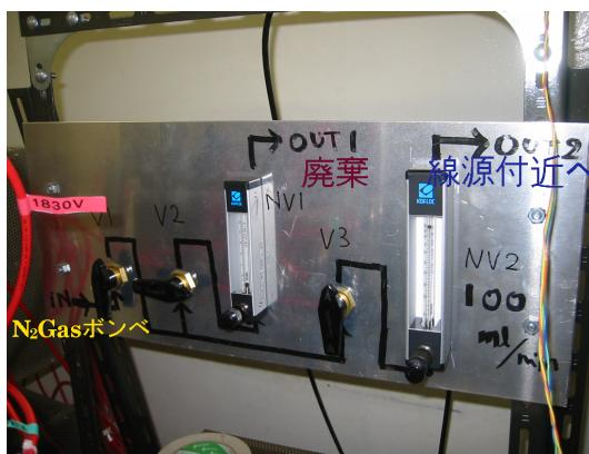
図 3.2: N<sub>2</sub> ガスの流れ
