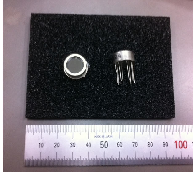
Figure 2.18: Pyroelectric detectors (Spectrum Detector Inc. SPH-49).
