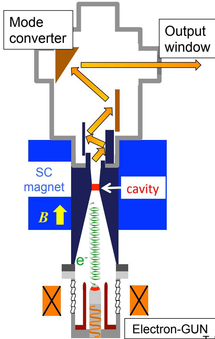
Gyrotron utilizes cyclotron motion of **electrons** to resonate a cavity inside the solenoid
