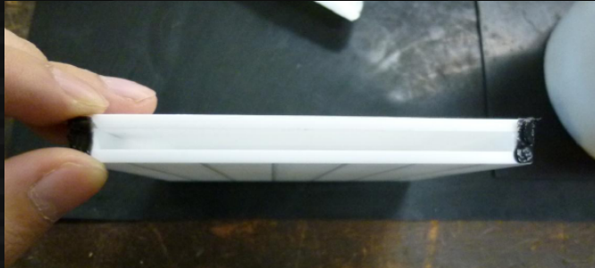
Water in a Teflon box for absolute calibration
