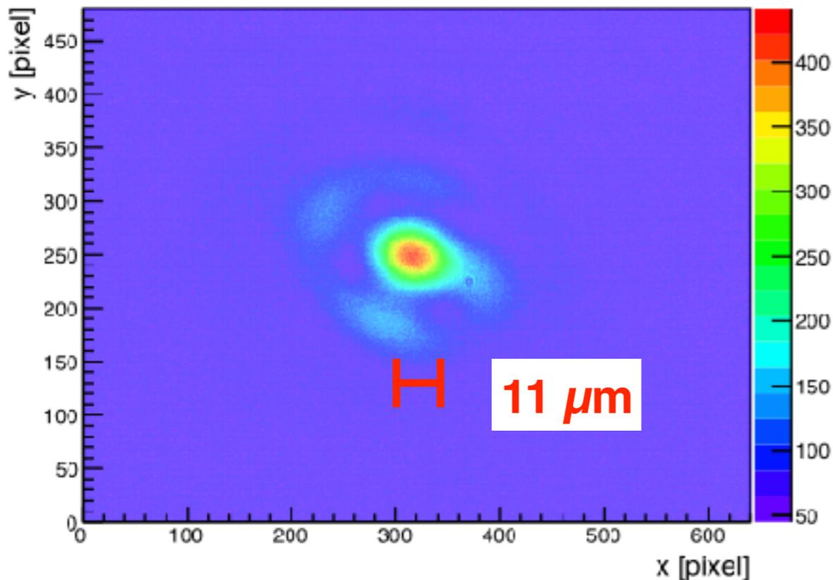
**Beam size of pump laser**
