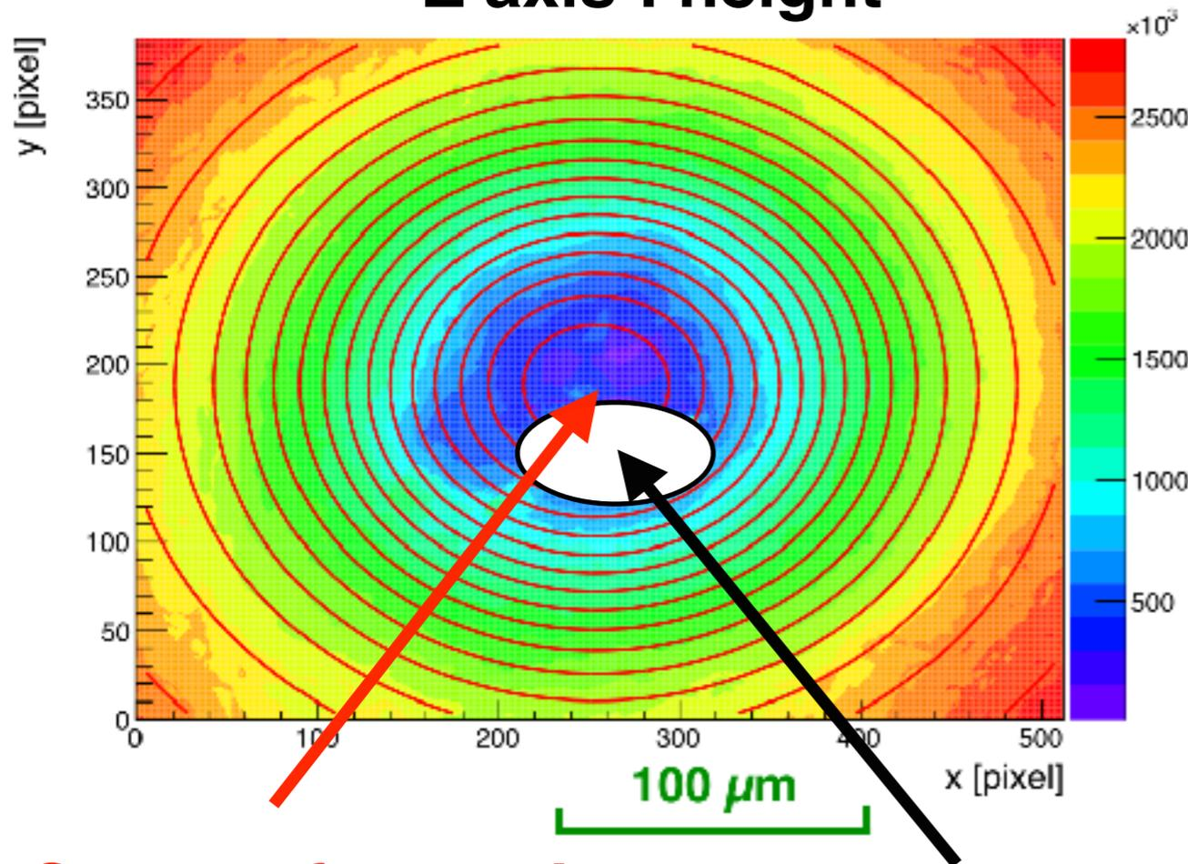
After beam time, I measured relative distance of irradiation traces using laser microscope.
