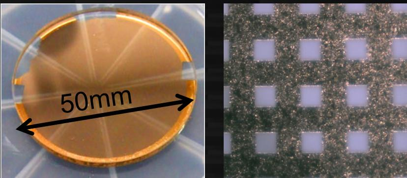
Au mesh (200 $\mu\text{m}$  width, 360 $\mu\text{m}$  period, 1 $\mu\text{m}$  thick) depleted on quartz or silicon
