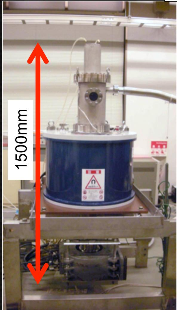
Gaussian beam converter
