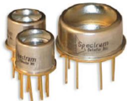
Pyroelectric detector is used to monitor transmission power of the cavity
