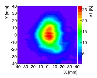
Figure 2.25: A picture of the PVC sheet taken by IR camera to estimate  $P_{\text{hole}}/P_{\text{in}}$ . The origin is the position of the hole at the center of the Cu concave mirror.
