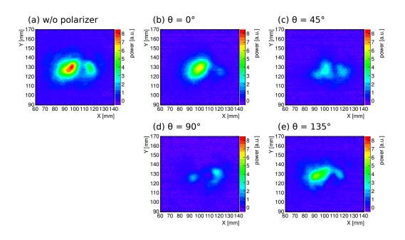
Figure 2.12: Polarization of the converted beam.  $\theta$  is the angle of the electric field from the horizontal direction.
