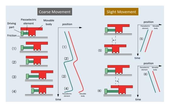
Figure 2.19: Principal of operation of an SIDM<sup>TM</sup> (Smooth Impact Drive Mechanism) actuator.
