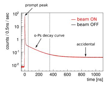
Figure 3.9: Time difference between the plastic scintillator and the coincidence signal of the  $LaBr_3(Ce)$  scintillators. Time window is set from 50 ns to 350 ns (black dash line). Note that this spectrum is a spectrum of the mean time of the two back-to-back  $LaBr_3(Ce)$  hits.
