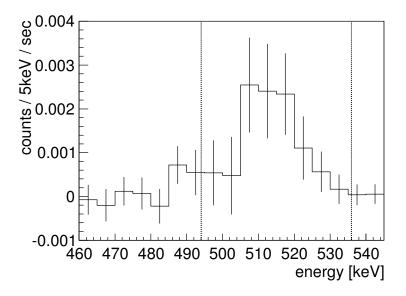
Figure 3.13: Energy spectrum of on-resonance data (RUN I) when the delayed coincidence and the accidental rejection are applied and a 511 keV  $\gamma$  ray is observed (energy window is set from 494 keV to 536 keV) at the opposite side of the LaBr<sub>3</sub>(Ce) scintillator. Accidental background estimated from the events in the time window set from 850 ns to 900 ns is subtracted. (top) ON (red line), OFF (black line), (bottom) ON – OFF
