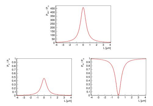
Figure 2.15: Basic performance of Fabry-Pérot resonant cavity calculated with  $R_{\rm f}=99.38~\%$ ,  $T_{\rm f}=0.39~\%$ ,  $R_{\rm e}=99.8~\%$ , and  $T_{\rm e}=0.2~\%$ . The top figure shows accumulated power, the bottom left figure shows transmitted power, and the bottom right figure shows reflected power.
