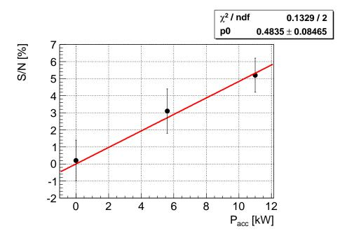
Figure 3.16: The fraction of the transition signals is proportional to the accumulated power in the Fabry-Pérot resonant cavity.
