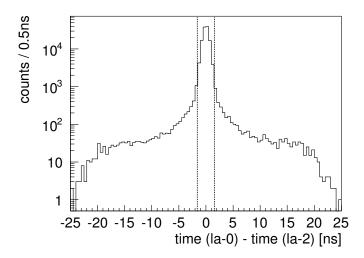
Figure 3.8: Time difference between the back-to-back signals from the  $LaBr_3(Ce)$  scintillators. The coincidence cut region is shown in black dash line.
