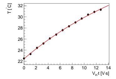
Figure 2.23: Temperature of water measured while the water is exposed to the Gaussian beam during 120 s. The horizontal axis of the figure is the integral of the input beam power measured with a pyroelectric detector.
