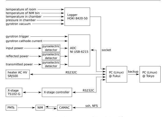
Figure 2.37: The schematic view of the whole DAQ system.
