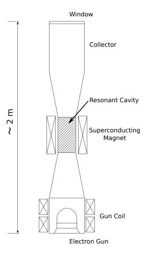
Figure 2.1: A schematic of a gyrotron.
