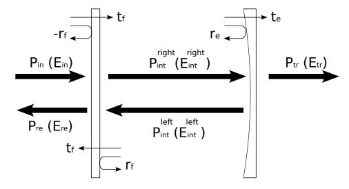
Figure 2.14: A schematic of a Fabry-Pérot resonant cavity.
