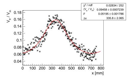
Figure 2.24: The transmitted power of the Cu concave mirror  $V_{\rm tr}$  normalized by the input beam power  $V_{\rm in}$  while changing the cavity length L by  $\lambda/2$ .
