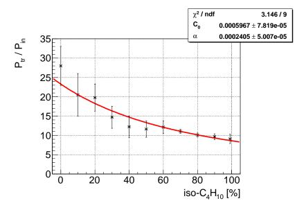
Figure 2.35: Absorption of sub-THz radiation by isobutane.
