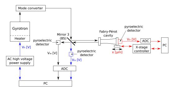
Figure 2.26: Schematic diagram of the feedback stabilization system. The feedback circuit for the gyrotron output power is shown in blue line. The red line shows the feedback circuit for the Fabry-Pérot resonant cavity stabilization.
