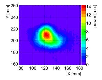
Figure 2.13: Beam shape after the mode converter.
