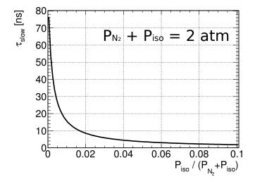
Figure 2.34: The lifetime of the slow positron as a function of the partial pressure of isobutane.
