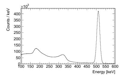
Figure 3.3: Energy spectrum of one of the  $LaBr_3(Ce)$  scintillators (la-0). The time window is restricted within prompt peak (from -3 ns to 1.5 ns).
