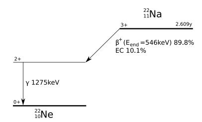
Figure 2.33: The decay scheme of the  $^{22}$ Na isotope
