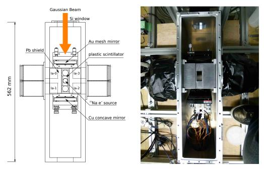
Figure 2.31: A schematic and a picture of the positronium assembly chamber and  $\gamma$ -ray detectors. The plastic scintillator and the <sup>22</sup>Na source is not placed in the right picture.
