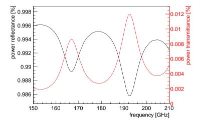
Figure 2.18: The reflectance (black) and the transmittance (red) of the Au plain mesh mirror simulated using CST MICROWAVE STUDIO.
