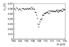
Figure 4.5: Interference between input power and reflected power around resonance peak. The left figure shows input power while changing the cavity length and the right figure is reflected power.
