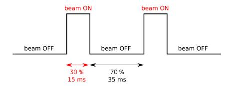
Figure 3.1: The timing diagram of the gyrotron output. The pulse frequency is 20 Hz and the duty ratio is 30 %.
