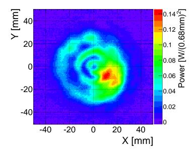
Figure 2.5: Space distribution of the gyrotron output (TE<sub>03</sub> mode).
