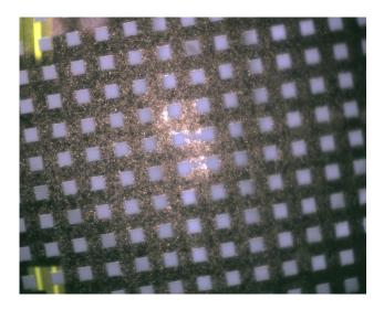
Figure 4.4: A picture of a melted mesh mirror.
