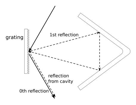
Figure 4.6: A schematic of a grating ring cavity.
