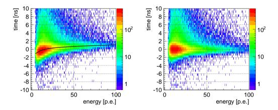
Figure 3.5: The left and the right figure show the scatter plot of timing vs energy deposited on the plastic scintillator before and after time walk correction, respectively.
