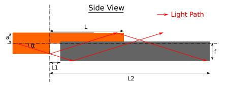
Figure 2.9: Side view of the step-cut waveguide and the Vlasov mirror
