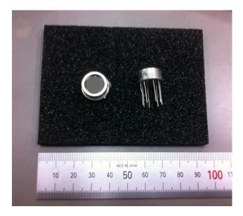
Figure 2.21: Pyroelectric detectors (Spectrum Detector Inc. SPH-49).
