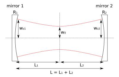
Figure 2.16: The beam shape in the Fabry-Pérot cavity.
