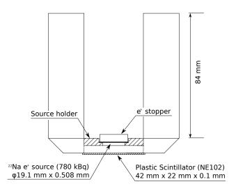
Figure 2.32: A schematic of the positronium formation assembly
