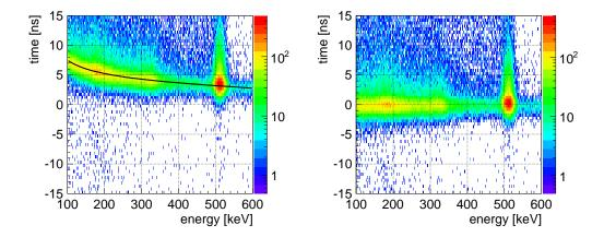
Figure 3.4: The left and the right figure show the scatter plot of timing vs energy deposited on one of the LaBr<sub>3</sub>(Ce) scintillators (la-0) before and after time walk correction, respectively.
