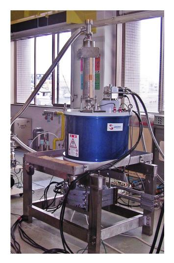
Figure 2.3: A picture of the Gyrotron FU CW V.
