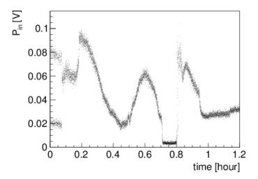
Figure 2.27: Time variation of the gyrotron output power is very large unless the feedback system is installed.
