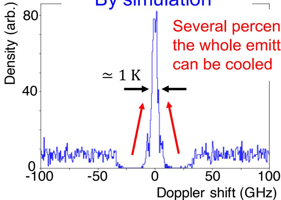
**Simulated Doppler shift after laser cooling by the prototypical laser**
