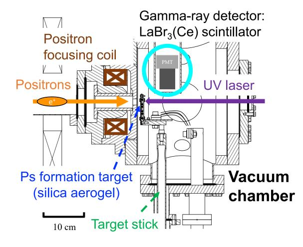
Positrons were focused to 3 mm so that it matched the laser size.
