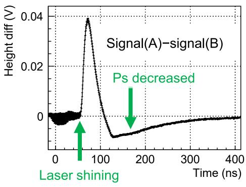
Signal difference caused by shining UV laser
