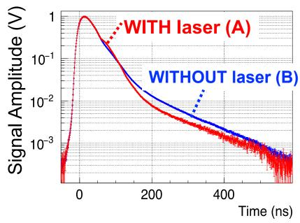
PMT signals made by annihilation gamma-rays detected by LaBr<sub>3</sub>(Ce) scintillator
