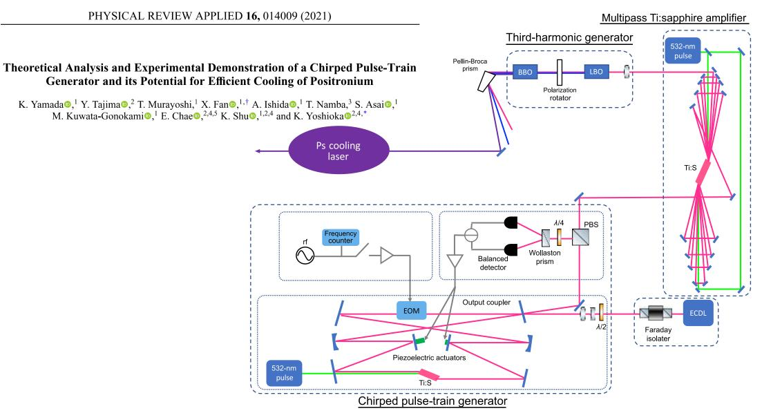
FIG. 1. Schematic of the prototypical cooling laser system. ECDL, external-cavity diode laser;  $\lambda/2$ , half-wave plate;  $\lambda/4$ , quarter-wave plate; EOM, electro-optic phase modulator; rf, driving radio frequency; Ti:S, Ti:sapphire crystal; PBS, polarizing beam splitter; LBO, lithium triborate crystal; BBO,  $\beta$ -barium borate crystal.
