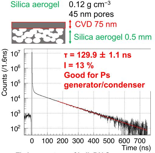
Timing spectrum of bulk-PALS measurement using <sup>22</sup>Na with t = 1 mm silica aerogel
