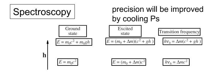
Fig. 1. Derivation of the gravitational red shift.
