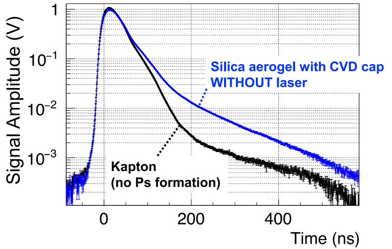
PMT signals made by annihilation gamma-rays detected by LaBr<sub>3</sub>(Ce) scintillator
