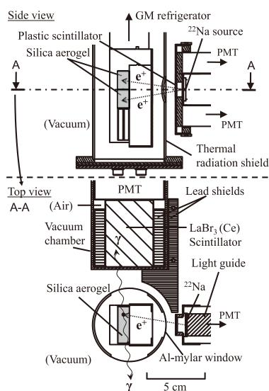
Observation of orthopositronium thermalization in silica aerogel at cryogenic temperatures
